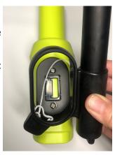
Stretch the rubber pole retainer around the lanyard section of the SART.
