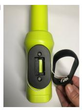
Carefully remove the lanyard end, which is located within the tab of the existing lanyard cover
